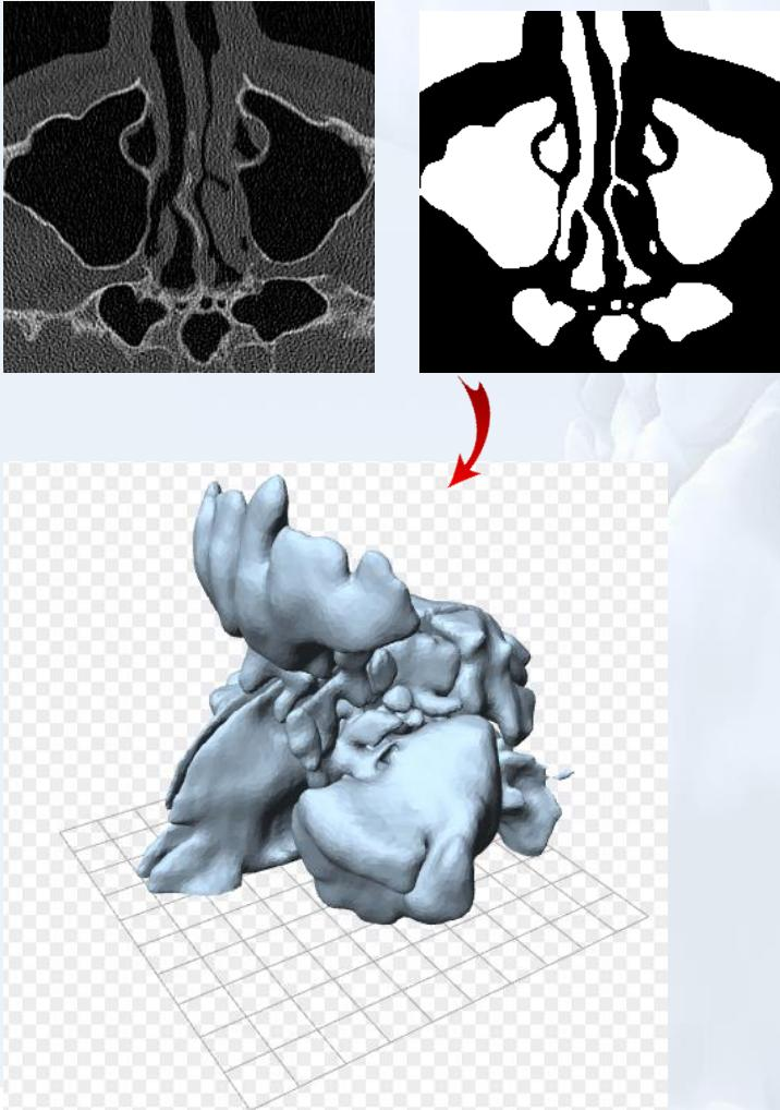
The **Marching Cubes** algorithm is used to extract polygonal mesh from an input isosurface. Using this algorithm, one can generate 3D surface triangulations, from the 2D segmentations of air and bone.
